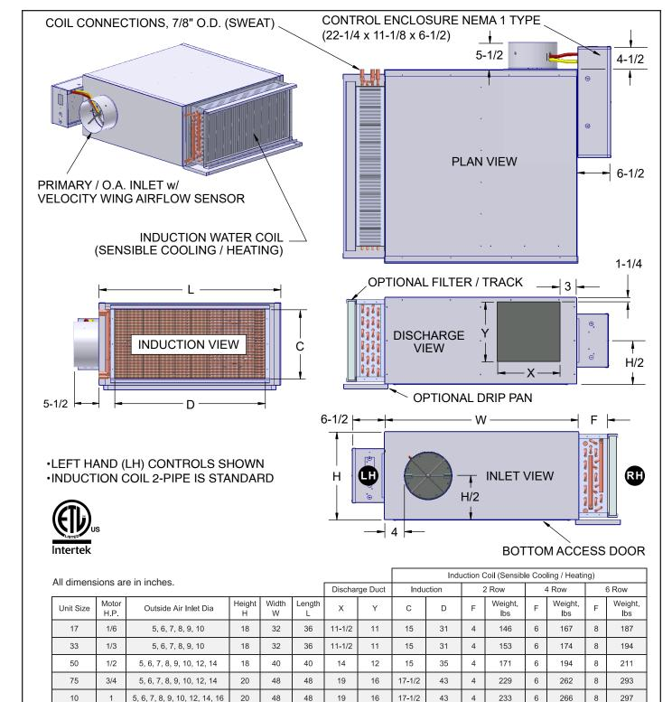
Weights are estimated totals and include coil fluid weight. Weights will vary with options & controls installed.
