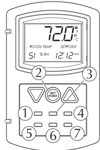
Each button of the NetSensor has an assignment for viewable and configurable variables in the VAV controller to which it is connected. These button assignments are clearly referenced in the chart below.
