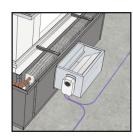
Model **RFCP-CI CONTINUOUS LINEAR PLENUM** INSIDE CORNER ASSEMBLY
