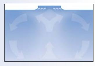
**90%+ ADPI** – The ADPI (Air Diffusion Performance Index) quantifies the percent of occupants within the space as thermally comfortable – higher is better. The HPX is better! More comfortable occupants means increased productivity and less time at the water cooler! Higher efficiency, reduced costs.
