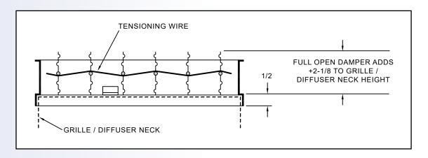
Dampers on this page are designed for low pressure adjustment of air flow, and are not intended for full shut-off applications. Contact your local Anemostat representative for details on full shut-off dampers.
