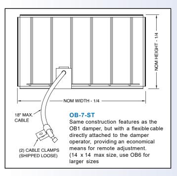
Dampers on this page are designed for low pressure adjustment of air flow, and are not intended for full shut-off applications. Contact your local Anemostat representative for details on full shut-off dampers.
