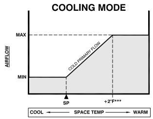
\*\*\* PROPORTIONAL BAND (**PROP BD**) DEFAULT AT 2°F, ADJUSTABLE FROM 1 to 10°F IN "ADVANCE" MENU ON THERMOSTAT
