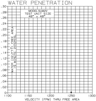
+ THE BEGINNING POINT OF WATER PENETRATION IS ABOVE 1250 FPM THROUGH THE FREE AREA OF THE LOUVER.
