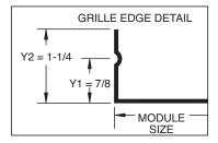
NOTE: Y1 & Y2 CAN BE MODIFIED FOR VARIOUS METAL PAN SYSTEM MANUFACTURERS
