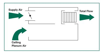
With this arrangement, the box fan air flow rate is the same as the supply air flow rate into the space:
